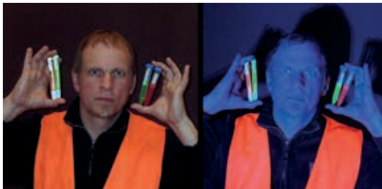
Fluorescence in action. Images show the fluorescence of high visibility clothing, marker pens and purified coral pigments under daylight (left) and under blue light (right).
